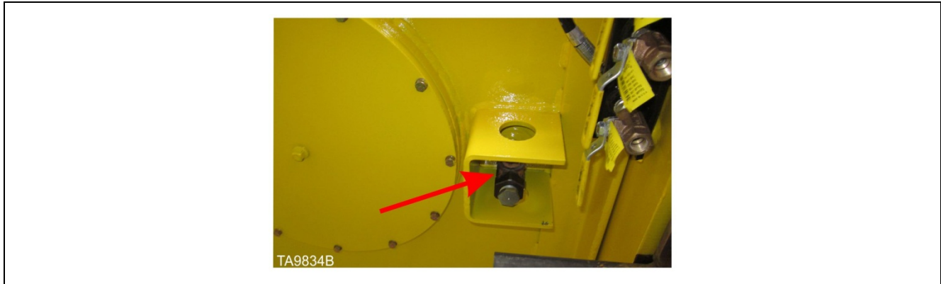
Figure 6. Hydraulic reservoir drain valve
