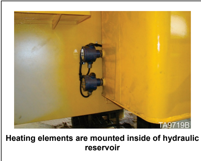
Figure 16. Hydraulic reservoir heaters (optional)
