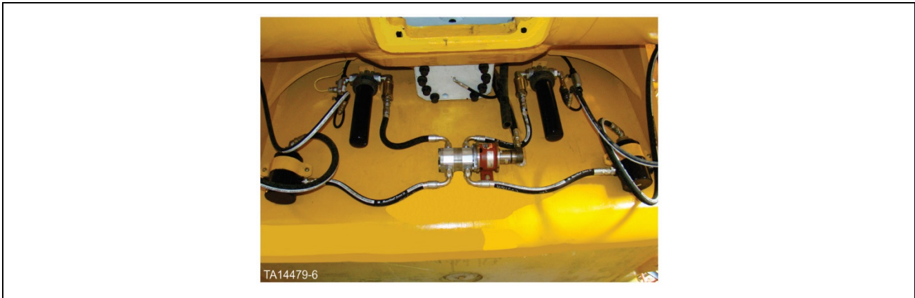
Figure 69. Rear planetary drive filtration system component mounting locations
