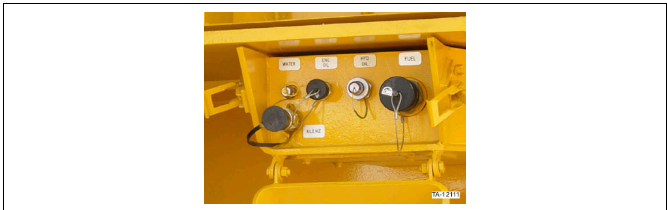
Figure 7. Central service system
